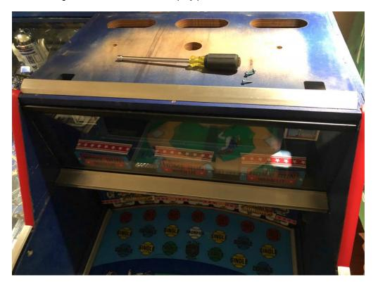
8. Carefully (without dropping them!) remove the 4 phillips head screws that secure the front display panel.
