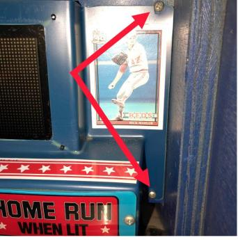
9. Remove the display panel to access the original factory DMD. You might have to lean the panel forward and push down a little on the top edge to ease it out.
