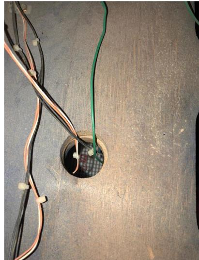
2. Standing at the rear of the machine, on the right side of the head, locate and remove the wingnut that secures the green ground wires. Remove the ground wire coming up from the lower head, and then replace the wingnut.
