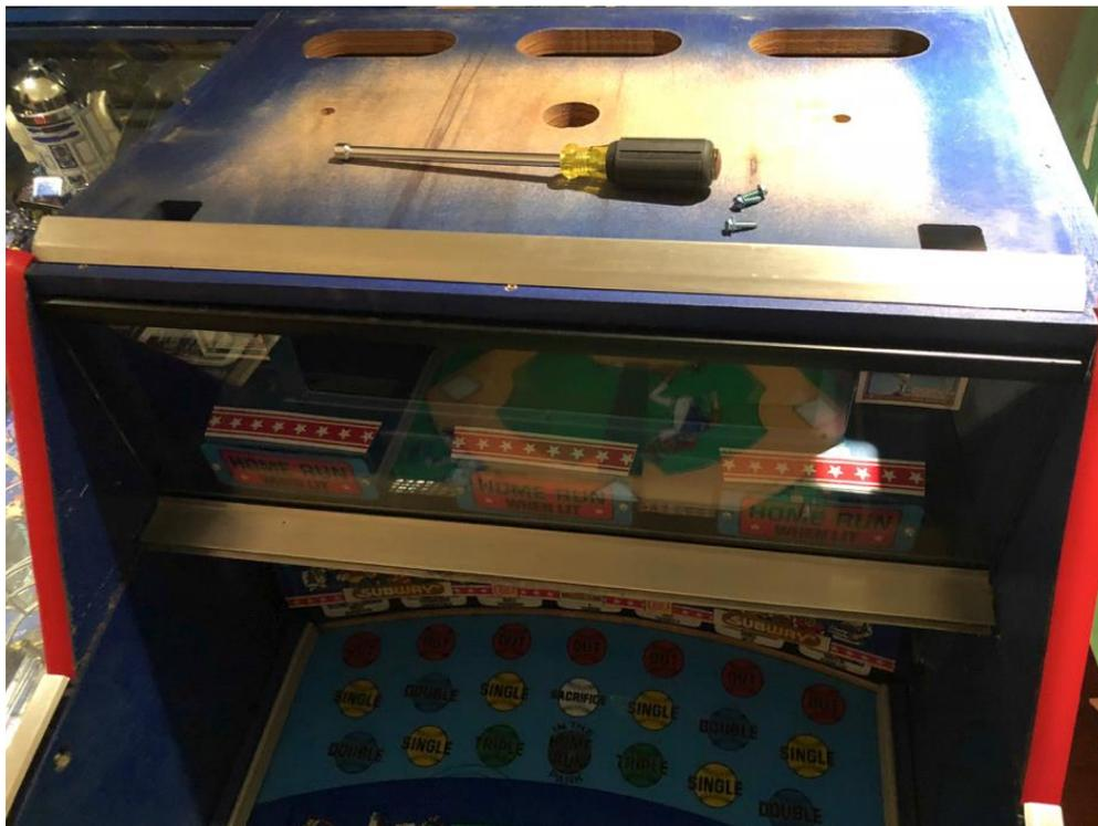
8. Carefully (without dropping them!) remove the 4 phillips head screws that secure the front display panel.
