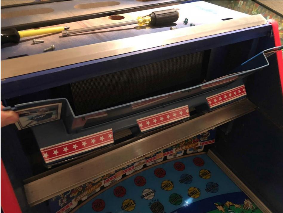
10. Remove the original factory DMD by gently pinching on the white nylon PCB standoffs and pulling the DMD forward.
